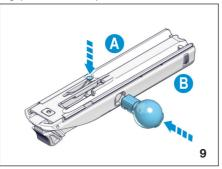
Refit the bolt head assembly into the carrier.
