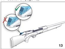
Proceed to fit the bolt carrier into the receiver: make sure the guides are correctly coupled.
