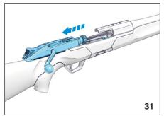
Move the carrier forward to chamber a cartridge.
