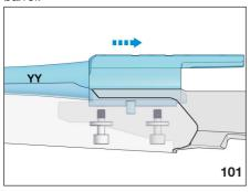
Refit the bolt carrier, making sure the guides are correctly coupled and that the bolt head is in the open position.
