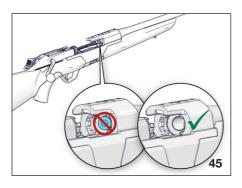
Press both release buttons and remove the magazine.
