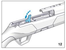
Make sure that the safety is NOT in the "carrier locked" position (see the "SAFE-TY" section on page 15).
