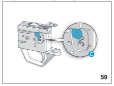
At the end of adjustment, make sure that the trigger latch is at the end of its travel, by pulling it upwards.
