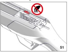
Gently press the safety and insert a flathead screwdriver into the trigger group latch to lift the latch itself.
