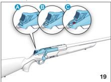
♠ Total lock position: carrier and trigger locked.
