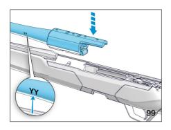
Tighten the fastening screws to a torque of 10Nm.
