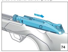
Slightly move the bolt carrier forward.
