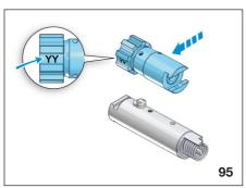
Loosen the two barrel fastening screws (7/32" mm Allen key).
