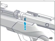
Slide the carrier out completely.
