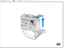
Before refitting the trigger housing, pull the trigger to release the hammer.
