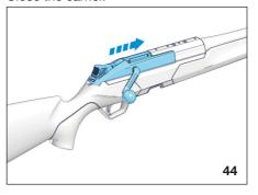
Move the carrier back to eject any cartridge from the chamber.
