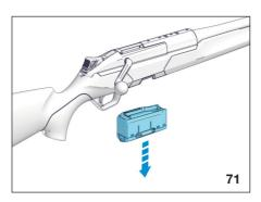
Slide the carrier out completely.
