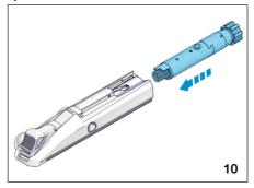
Check the barrel. The barrel and cartridge chamber must be clean and free from obstructions (see "Obstruction Check" on page 10).
