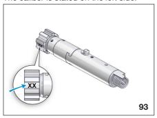
Fit the new caliber bolt head taking care to face the ejection port the right way (see the "ASSEMBLY" paragraph on page 10).
