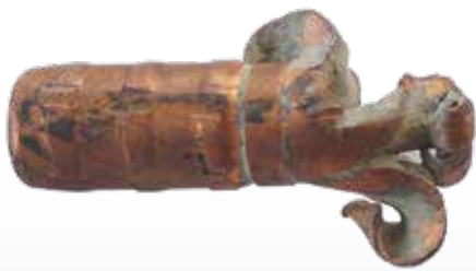
Bullet LFB COMPACT deformed
