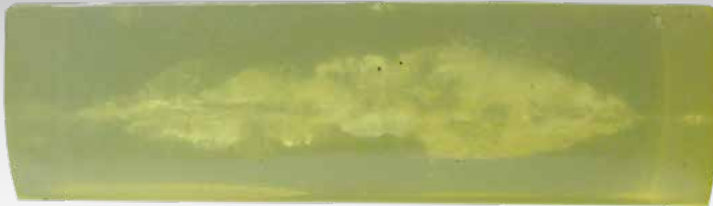
Practical test: shot into a gelatin block
