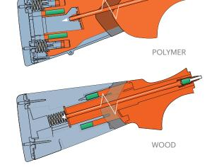
**Kick-Off® Plus** consists of two elastomer shock absorbers, positioned close to the rubber insert and equipped with return springs, which effectively act on the first recoil peak, reducing its perception up to 40%. A third elastomer shock absorber, inserted in the tie rod, absorbs the impact of the slide against the receiver, reducing the second recoil peak, the muzzle rise effect and the vibrations caused by the movement of the slide.
